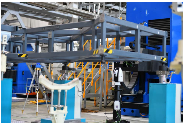
图5 大部件对接工艺试验 Fig.5 Butt joint process test of large parts
