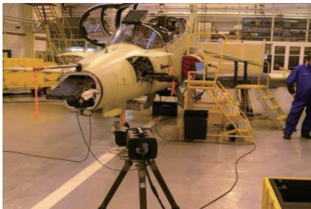
图6 校靶过程的数字化测量 Fig.6 Digital measurement of target calibration process
